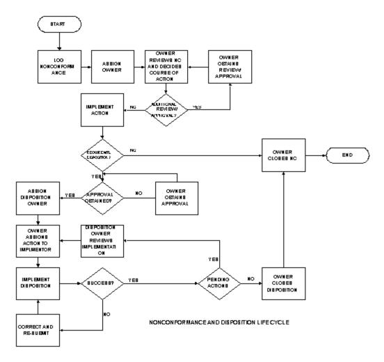
Figure 2–5 Nonconformance and Disposition Lifecycle
