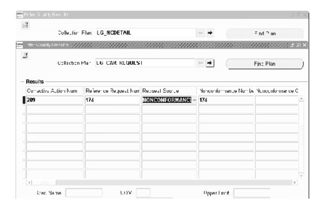
Figure 12–14 Entering a CAR with Nonconformance as Request Source
